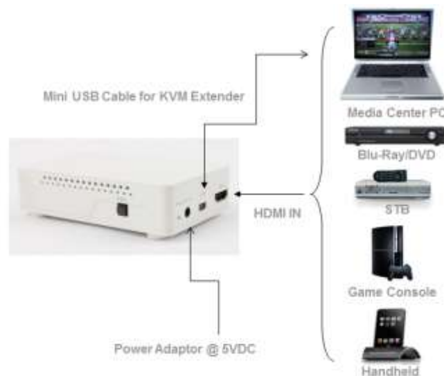
Fig. 1: Configuration of Transmitter, HDWX-100-T
